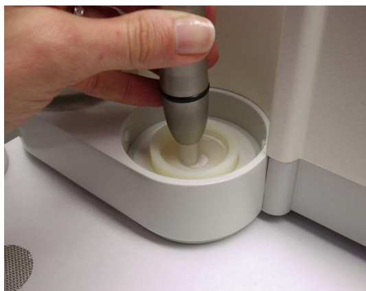
Fig. 29: Suck off the crystal sand
