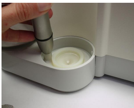
Fig. 31: Suck off the whole surface
