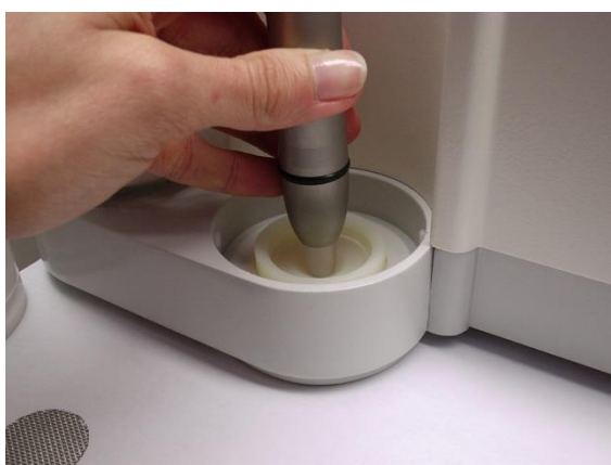
Fig. 30: Suck off the funnel opening
