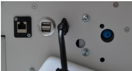
Fig 36. Port for USB stick on the underside of the device body
